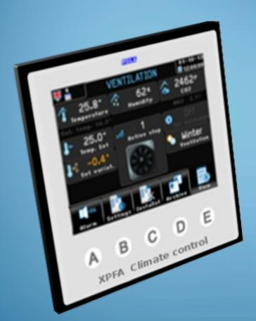
The main feature of the XPFA is the color display screen (3.5") with 320x240 dots resolution with led backlighting. XPFA is made in DIN 96x96 format and the module dimensions are 96x96mm.
