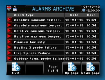
Recording all the alarm events for temperature, humidity, air-pressure, C02-NH3, including alarm exclusions. Archives contain all alarms triggered during current cycle.
