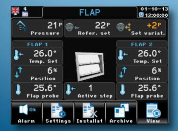
Up to 2 independent flaps (air inlets) working either by static pressure by Depressiometer or Associative or Proportional or Natural mode (by 0-10V or by feedback potentiometer).
