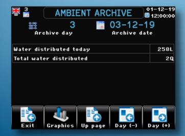
Water consumption is recorded by the CWD water meter.
